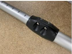
Mount the lever and tighten the bolts lightly, you will see there is a bigger gap on the replacement base clamp.
