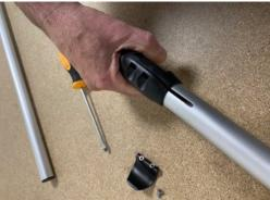
Open the clamp with a screwdriver and pull off the base clamp
